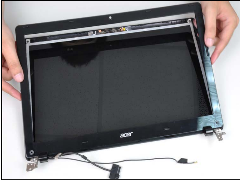
Figure 3-44. LCD Bezel Removal
