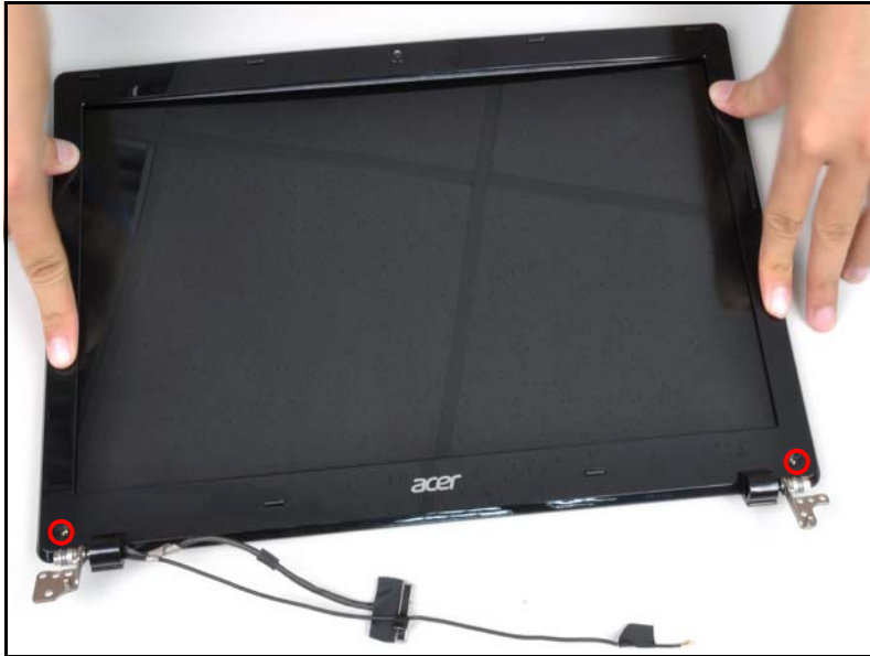
Figure 3-42. LCD Bezel Screws
