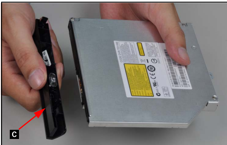
Figure 3-9. ODD bezel Removal
