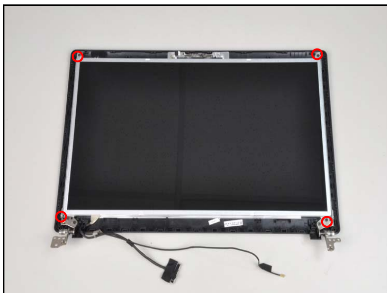
Figure 3-48. LCD Panel Screws
