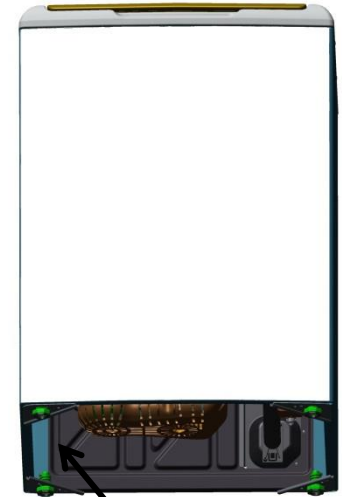
The mini (maxi) manual location. Tilt washer back to retrieve.
