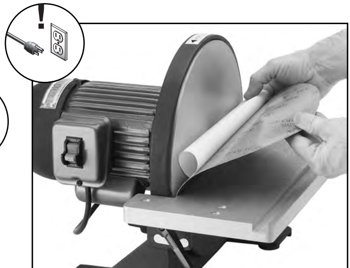
Figure 5. Sandpaper being slipped between the disc and table.
