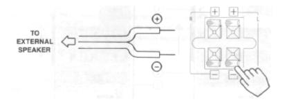
**CAUTION:** Do not connect Speakers simultaneously to the REAR SPEAKER terminal of the Projection TV and Amplifier. This could damage both the Projection TV and the Speakers.
