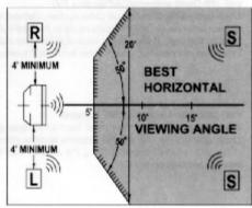
**NOTE:** The magnetic field of external speakers may cause the TV picture to distort if the speakers are placed too close to the television. Move the speakers away from the TV until there is no picture distortion.
