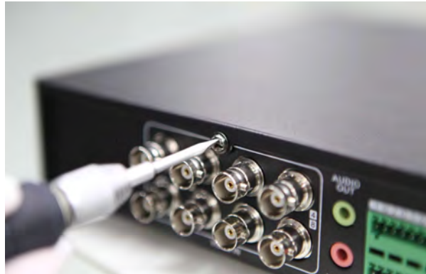
Figure 1 Removing the Cover
