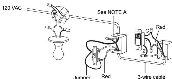
Connect wire "C" of the RPLS530A/RPLS531A to the "common" wire, identified when removing the old switch. Connect the other two RPLS530A/RPLS531A wires to the two remaining wires.
