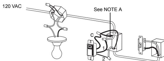
The jumper wire is not required in this installation. A single-pole switch can be used as the other switch in a 3-way installation.
