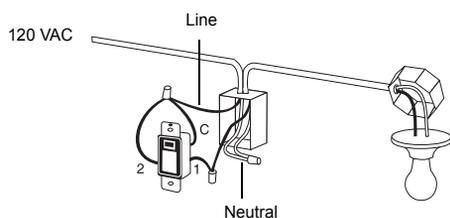
Connect wires "2" and "C" of the RPLS530A/RPLS531A to the line (120 V) wire.
