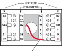
For 24VAC primary power, connect common side of transformer to "C" terminal.
