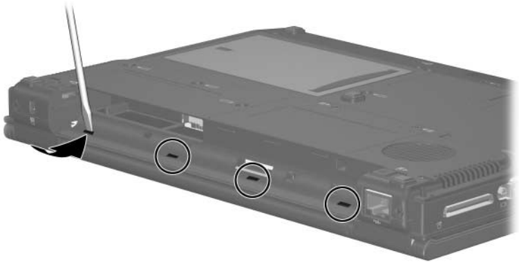
Releasing the Switch Cover, Part 1
