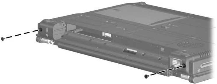
Removing the Display Assembly Screws
