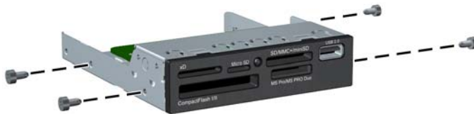
Figure 7-20 Installing Guide Screws (Media Card Reader Shown)
