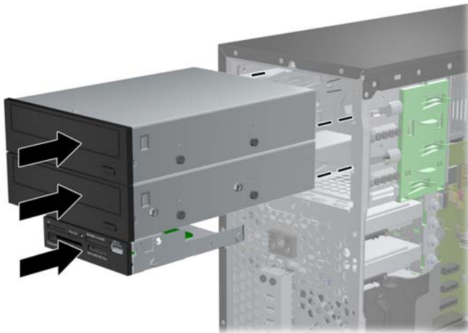
Figure 6-18 Sliding the Drives into the Drive Cage
