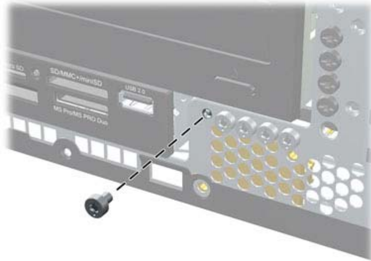
Figure 7-3 Retrieving the Front Bezel Security Screw
