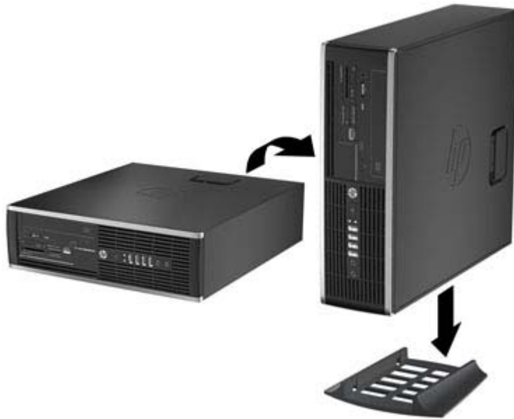
Figure 7-40 Changing from Desktop to Tower Orientation
