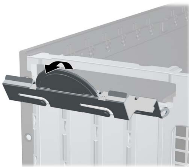
Figure 7-7 Opening the Expansion Slot Retainer
