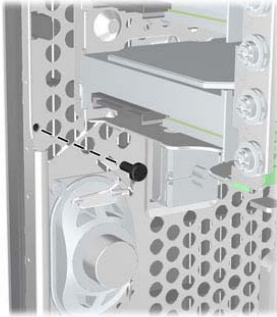
Figure 6-4 Installing the Front Bezel Security Screw
