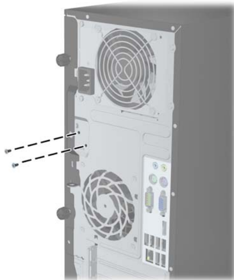
Figure C-2 Removing the Smart Cover Lock Screws from the Microtower
