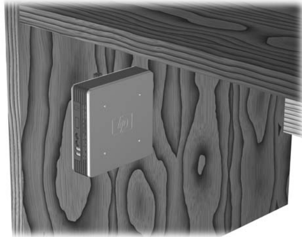
Figure 5-8 Thin client mounted under desk
