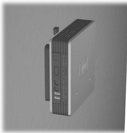
Figure 5-7 Thin client mounted on wall
