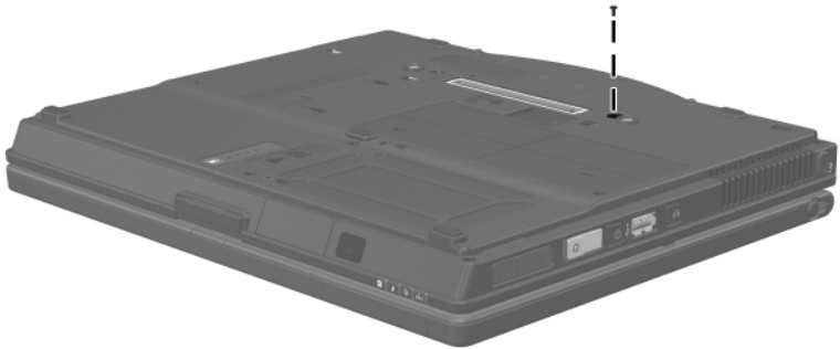
Torx8 T8M2.0x5.0 Screw Location
