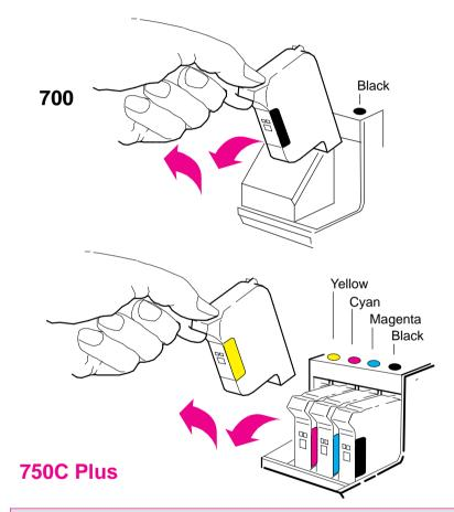
Notice that each stall in the carriage has a dot indicating the color: when loading the new cartridge you *must* put the correct cartridge in the correct stall.
