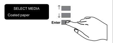
If you are using software that offers a "special print mode" for this plotter, then simply press **Enter** on the first media type displayed (whatever it is), as in this case it is the software that controls the print mode, not the plotter. For more details on special print modes, see page 3-6.
