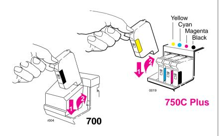
3 When the cartridges are successfully installed, the plotter automatically runs the cartridge alignment procedure. When the front-panel displays STATUS / Ready, the procedure is complete. You can throw away the small print produced during the cartridge alignment procedure.
