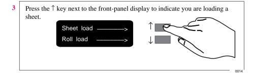
Press the ↑ or ↓ key until the display shows the type of media you are loading (if you are using regular plotter paper, scroll to Opaque bond; if coated paper, scroll to Coated paper), and then press the Enter key.
