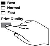
If you are using one of the software drivers supplied with the plotter, you can also make this setting (or an equivalent) within the driver. In this case, the driver setting will override the front-panel setting. The front-panel setting will, however, remain available as the default value, and the front-panel light displayed will not change.
