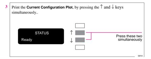
Notice on the Current Configuration Plot that the 16 pens are numbered 0 through 15.
