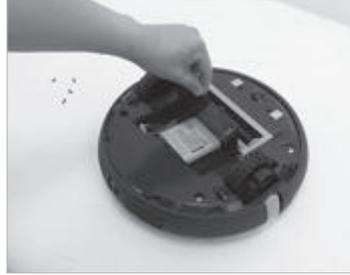
03. Pull out the battery pin and remove the battery.
