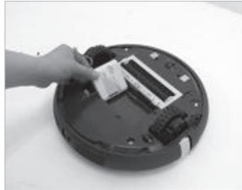
04. Replace with the new battery and insert the battery pin.
