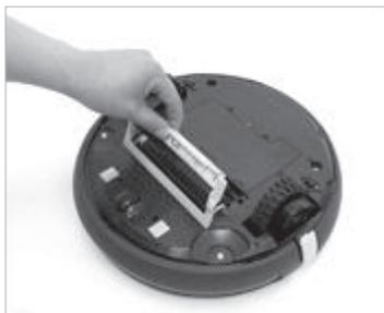
02. Remove the main brush by holding and lifting it.
