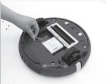
05. Close the battery cover and tighten the screws.
