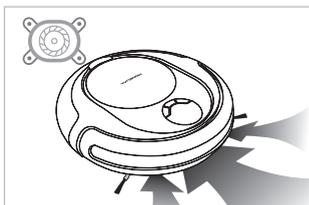
Cleaning capability is maximized through use of the powerful BLDC (suction) motor. The BLDC motor has 20~30% stronger output than that of a regular DC motor of the same class and also has the lifetime of approximately 5,000 hours, 10 times longer than that of a typical DC motor.
