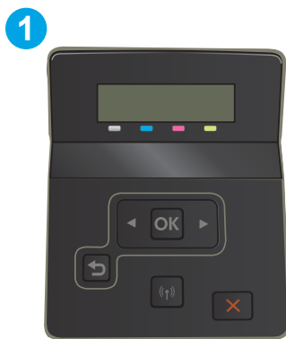
1 2-line control panel
