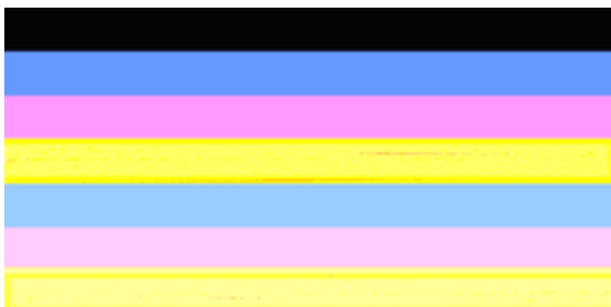
Print quality bars are not uniform The bars have lighter or darker portions in them.
