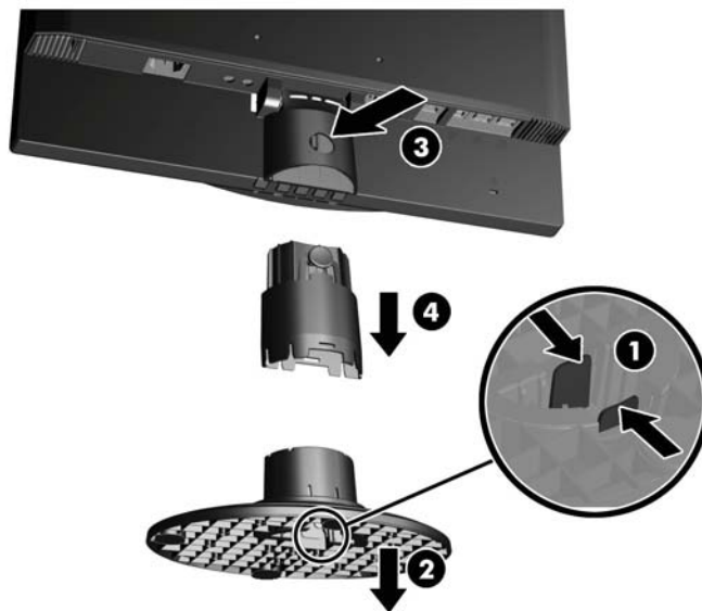
Figure 2-2 Removing the Monitor Center Column and Base
