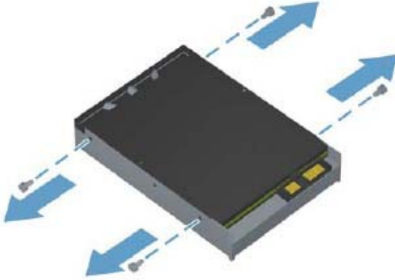
Figure 8-22 Removing the hard drive guide screws
