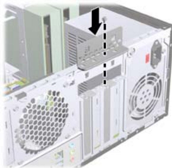
Figure 7-12 Securing the Expansion Cards and Slot Covers
