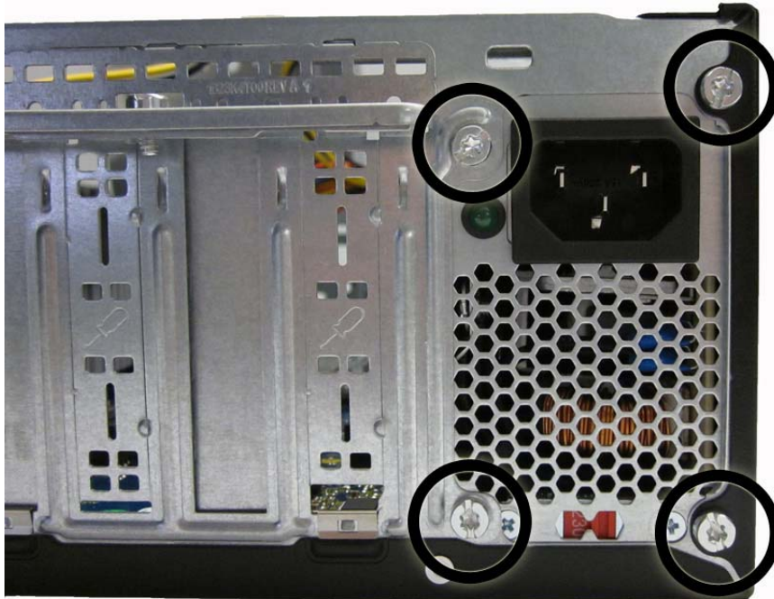
Figure 8-35 Removing the power supply screws
