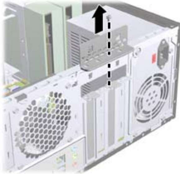
Figure 7-7 Opening the Slot Cover Lock
