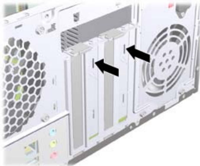
Figure 7-8 Removing an Expansion Slot Cover
