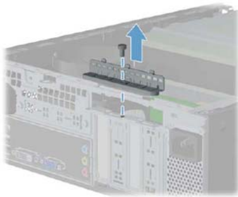
Figure 8-10 Opening the expansion slot bracket
