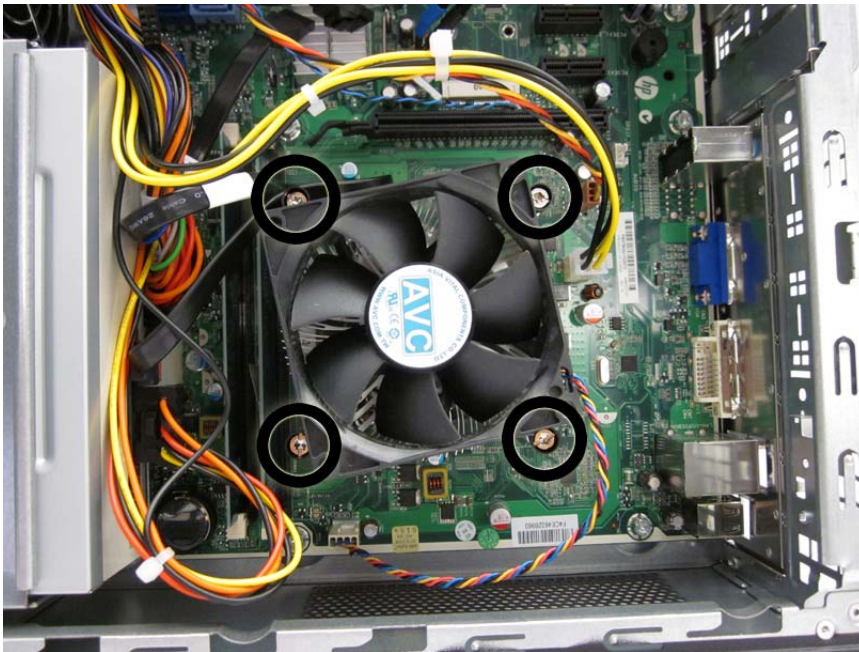
Figure 8-32 Loosening the fan sink screws
