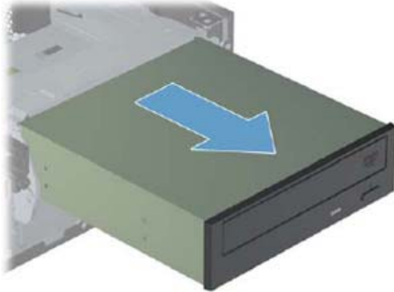
Figure 8-17 Removing the optical drive
