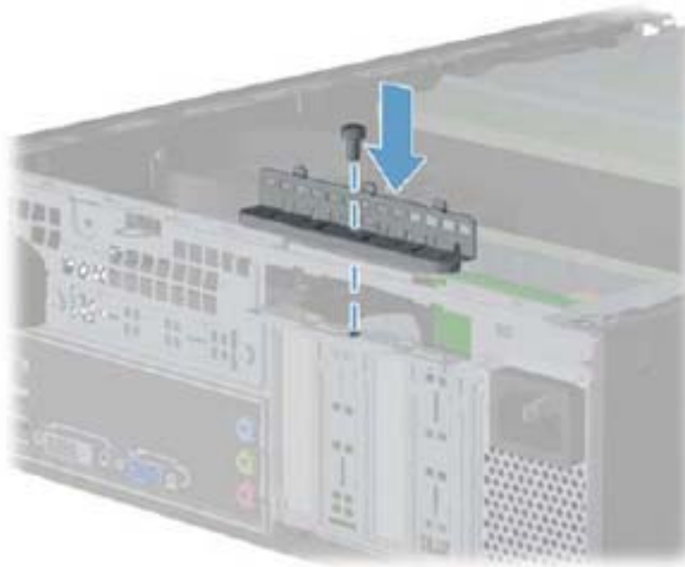
Figure 8-13 Replacing the expansion slot bracket
