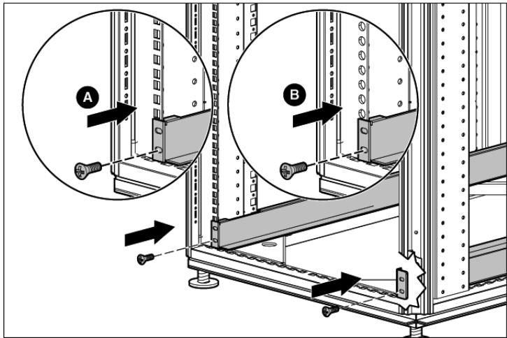
7. Tighten the wing nuts or hex nuts.
