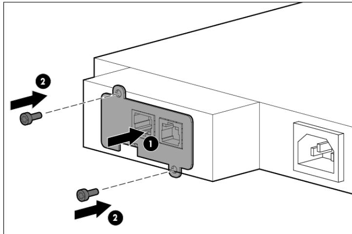
3. Secure the UPS Network Module using the two screws you removed in step 1.
