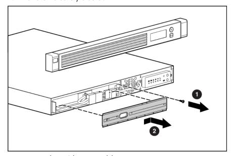
Remove the UPS battery modules.
