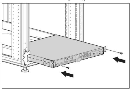
(optional) Insert the rear stabilization brackets into the mounting rails and then attach the brackets to the UPS.
