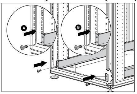
Tighten the wing nuts or hex nuts.
