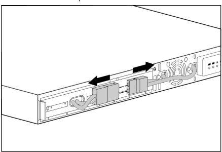
Remove the battery bracket.
