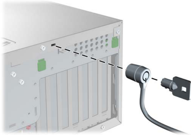
Figure 5-2 Removing the cable lock
