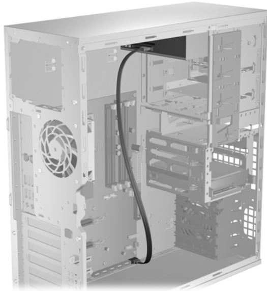
Figure 5-14 Connecting power and data cables
