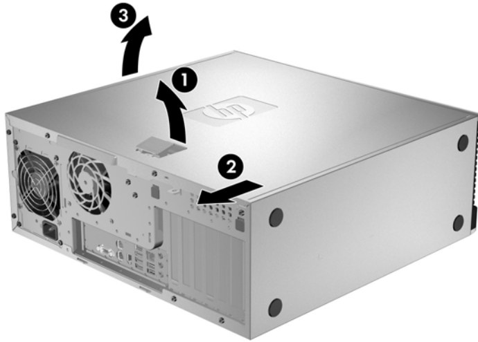
Figure 5-3 Removing the side access panel
