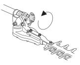
Press the cutting unit against the hedge or some other firm surface until the required angle is set.
