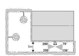
Area: 0.17 acre (700 m²). U-shaped garden with the charging station placed on one of the large open areas. Guide wire recommended through the passage.
