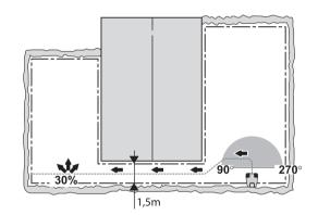
Area: 0.20 acre ( $800 \text{ m}^2$ ). Rectangular garden with the charging station placed by an island. A large part of the boundary wire is routed on a slope that is steeper than 10 %. Guide wire recommended.
