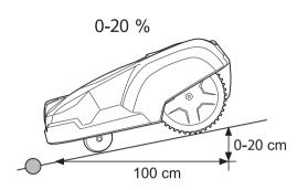
The boundary wire should not be laid across a slope that is steeper than 20 %. There is a risk of Automower® finding it difficult to turn there. The mower will then stop and show the fault message Outside working area. The risk is at its greatest in damp weather conditions, as the wheels can slip on the wet grass.
