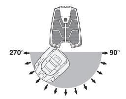
The mower can be set for up to two exit sectors. If the charging station is placed in a passage it may be necessary to have two exit sectors, e.g.  $70^{\circ}$  -  $110^{\circ}$  and  $250^{\circ}$  -  $290^{\circ}$ .
