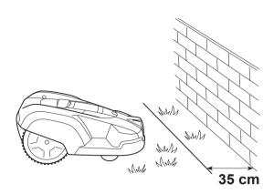
If the working area borders against a small ditch, for example, a flower bed or a small elevation, e.g. a low verge (1" - 2")((3 - 5 cm), the boundary wire should be laid 12" (30 cm) inside the working area. This prevents the wheels from driving into the ditch or up onto the verge.
