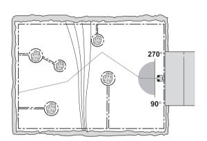
Area: 0.15 acre (600 m²). L-shaped garden with the charging station placed in the large open area. No guide wire is necessary.
