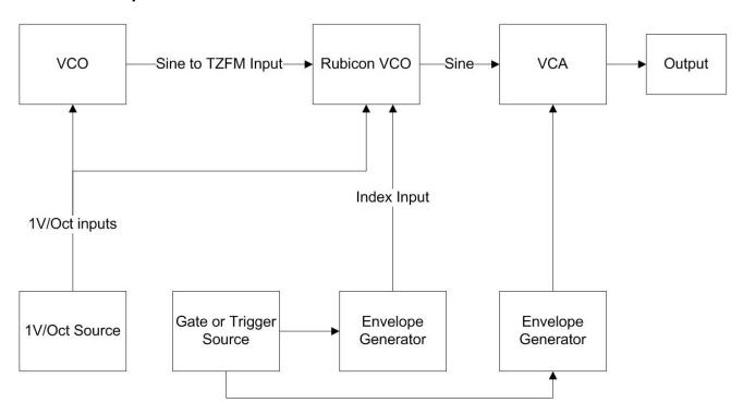
This is the most basic FM patch and is known as "Two Operator FM". It uses The Rubicon, another VCO, two Envelope Generators and a VCA. In FM terminology the Rubicon becomes the Carrier and the second VCO is the Modulator. Because they have similar pitch tracking we recommend the second VCO be a Intellijel Dixie or another Rubicon. You will need a 1V/oct and gate source such as a CV keyboard or MIDI to CV converter.
