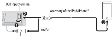
**KW-R935BTS**: You can also connect to the USB cable from the rear of the unit.
