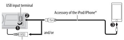
KW-R935BTS: You can also connect to the USB cable from the rear of the unit.
