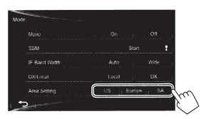
[US] Select this when using in North/ Central/South America. FM/AM intervals are set to 200 kHz/10 kHz.
