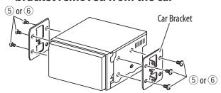
Select the appropriate type of screw for the mounting bracket: flat head (⑤) or round head (⑥).
