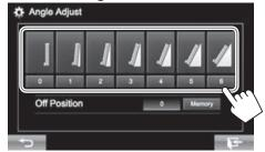
• To set the current position as the power off position, select [Memory] for <Off Position>.
