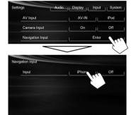
When <Input> is set to [iPhone], the [Apps] button is shown on the <**HOME**> screen, and the  $[\mathcal{A}]$  button is shown on the source control screen. You can display the App screen by pressing either button. (See the right column.)
