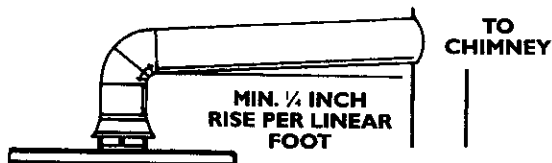
VENT PIPE INSTALLATION
