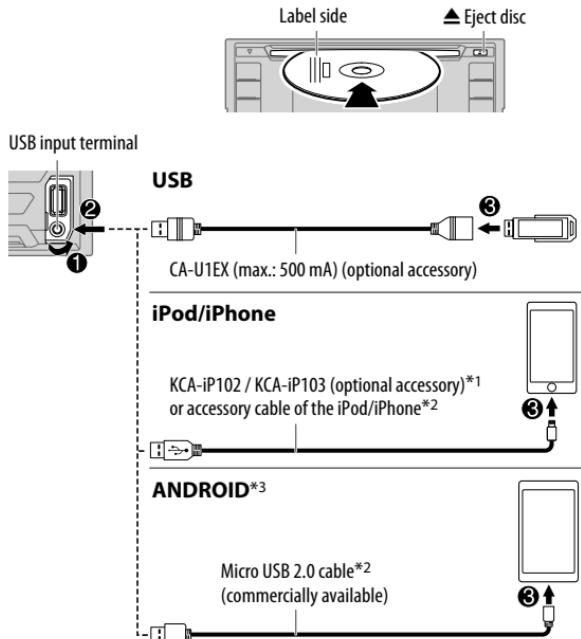
\*1 KCA-iP102 : 30-pin type, KCA-iP103 : Lightning type
