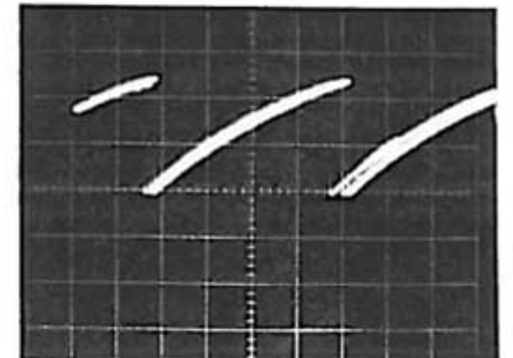
5 mS/cm, .1V/cm DC coupled: Confirm S-V converter operation
