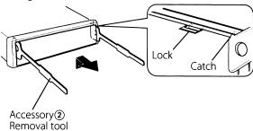
2 When the upper level is removed, remove the lower two locations.
