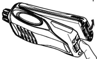
3 While pressing the release latch, pull the battery pack away from the transceiver.
