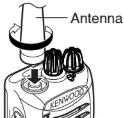
Screw the antenna into the connector on the top of the transceiver by holding the antenna at its base and turning it clockwise until secure.
