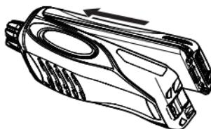
1 Align the battery pack with the back of the transceiver, then press the battery pack and transceiver firmly together until the release latch on the base of the transceiver locks.
