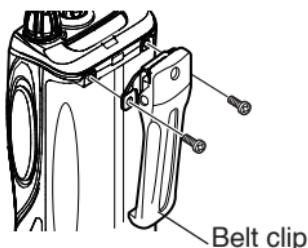
If necessary, attach the belt clip using the two supplied M3 x 8 mm screws.
