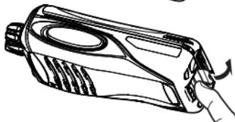
2 To remove the battery pack, lift the safety catch on the base of the transceiver, then press the release latch underneath the safety catch.
