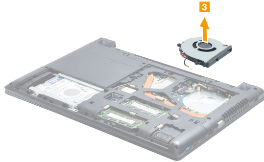
Figure 7. Removal steps of fan assembly (continued)
