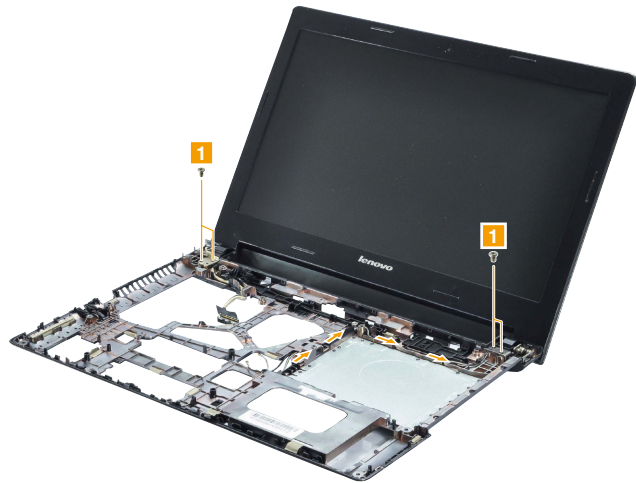
Figure 14. Removal steps of LCD unit
