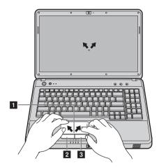
**Touchpad**To move the cursor on the screen, slide your fingertip over the pad in the direction in which you want the cursor to move.
