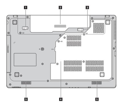
**Battery latch -** The manual battery latch is used to keep the battery pack secured in place.
