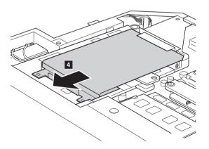
Take out the hard disk drive secured in a metal frame 5.
