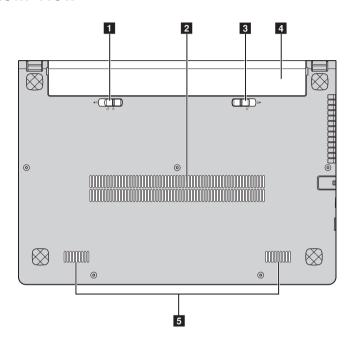
Battery latch - manual battery latch is used to keep the battery pack secured in place.
