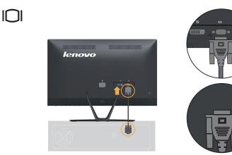
4. Connect the digital cable to the DVI connector of the monitor and the other end on the back of the computer.
