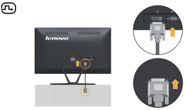
5. Insert the Adapter into the monitor, then plug the monitor power cord and the computer cord into grounded electrical outlets.
