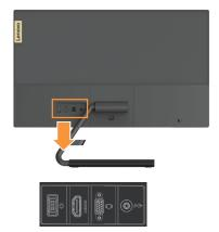
3. Connect one end of the HDMI cable to the monitor HDMI connector and the other end to the computer.
