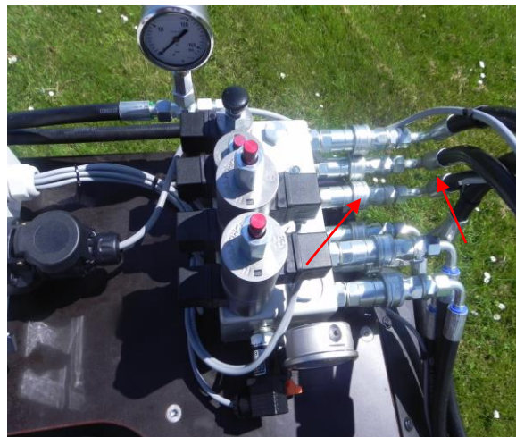
The numbers on the hoses and the numbers on the hydraulic block must match and be connected accordingly.
