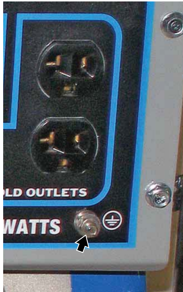
Figure 19 – Ground Terminal on the Control Panel
