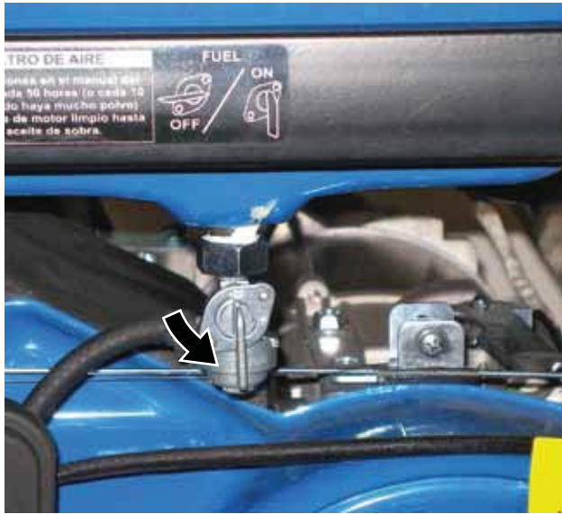
Figure 22 – Fuel Shutoff Valve in the ON Position
