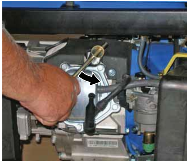
Figure 40 – Removing Spark Plug
