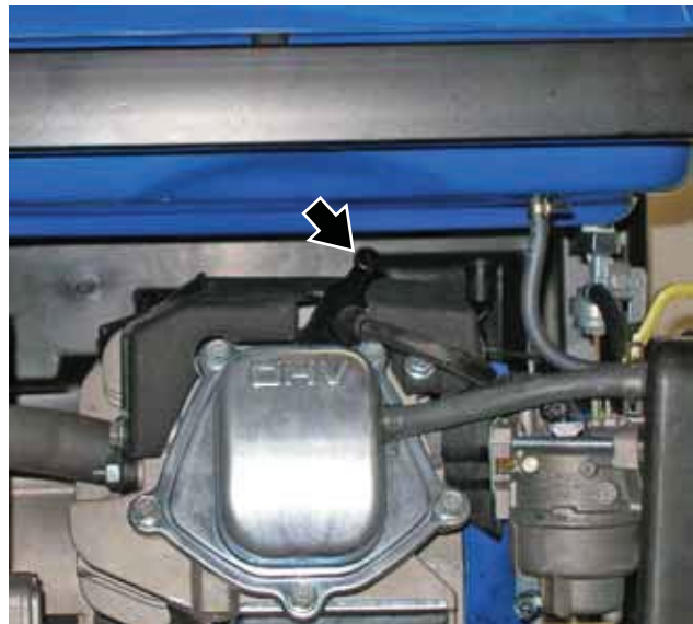
Figure 39 – Removal of Spark Plug Boot
