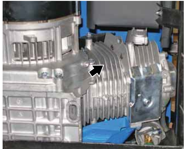
Figure 45 – Engine Cooling Fins
