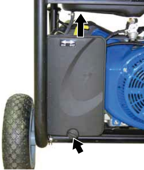
Figure 35 – Removing Air Cleaner Cover
