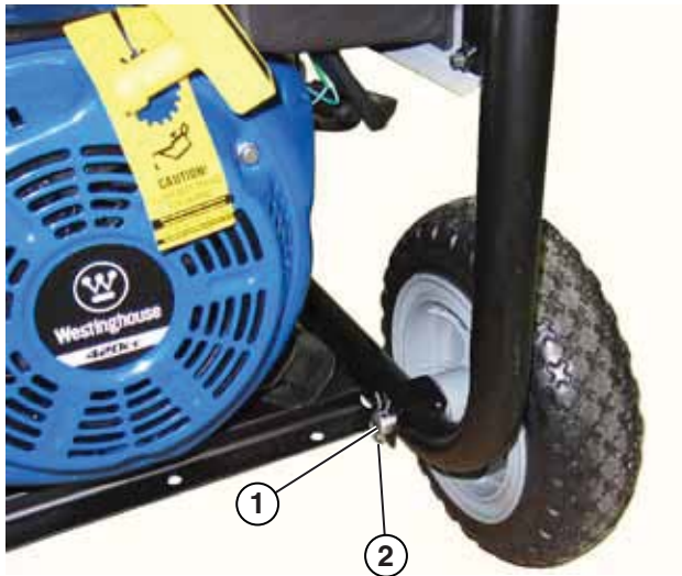
Figure 13 – Assemble Wheels to Frame
