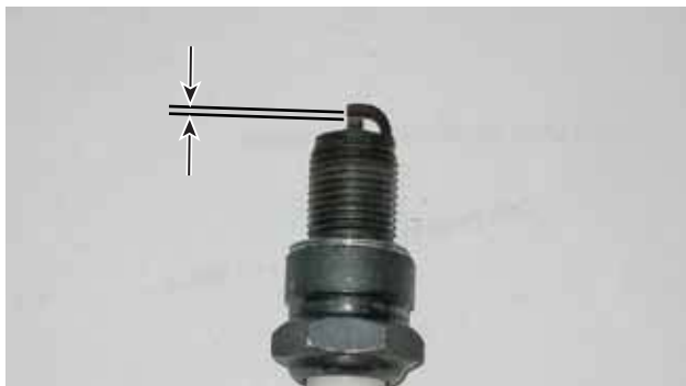
Figure 41 – Spark Plug Gap Requirements
