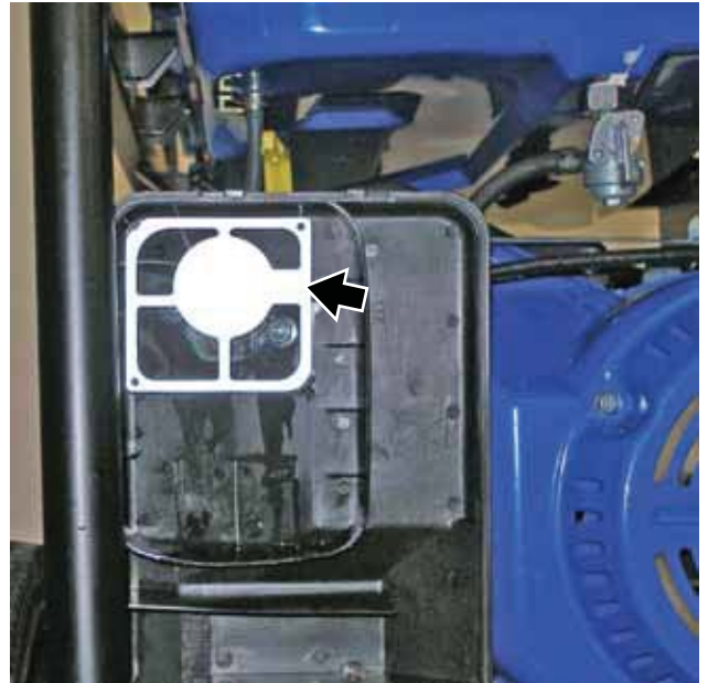
Figure 37 – Position of Metal Backfire Plate
