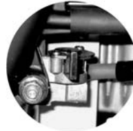
Fuel shutoff valve closed.
