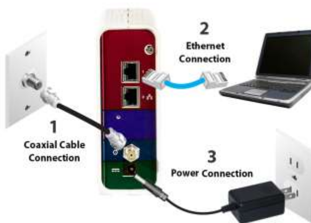
Figure 4: SBG6700-AC Connection Diagram
