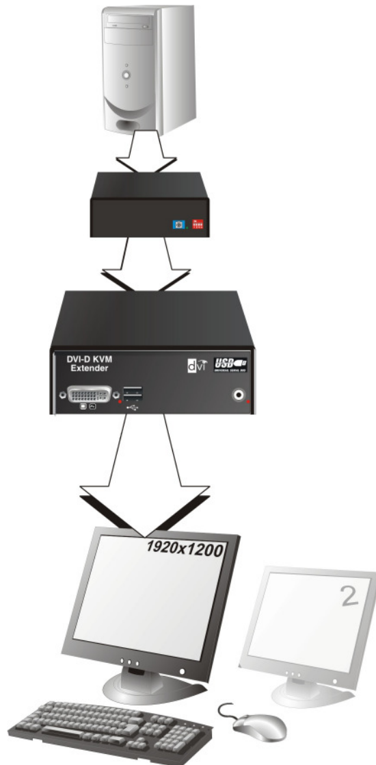
ACS1xxA KVM- (Singlelink-) Extender with optional, second screen.
