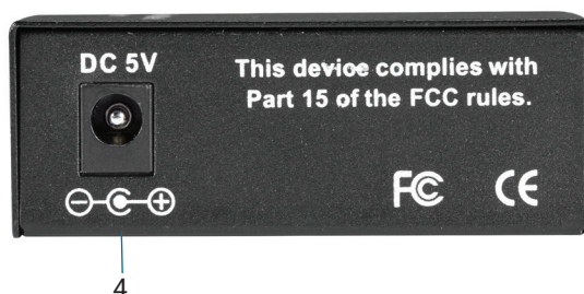
FIGURE 2-12. LGC212A BACK PANEL
