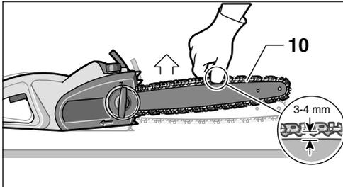
6. If the chain **10** is overtensioned, turn tensioning ring **13** anticlockwise to loosen the chain.
