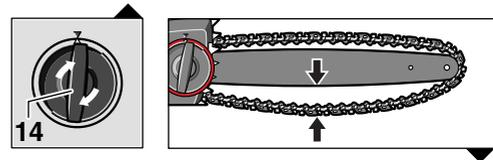
The chain is not yet tensioned. Tensioning the chain applies as described under "Tensioning chain", item 1–7.
