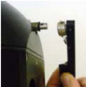
Figure 2.6: Remove Wiper Arm from wiper shaft
