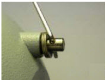
Figure 2.10: Replace 3 washers on shaft
