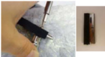
Figure 3.2: Replace Wiper Blade
