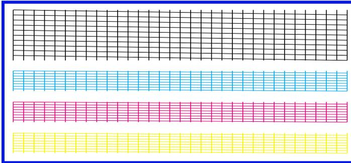
Lines missing here indicate the print head requires cleaning.
