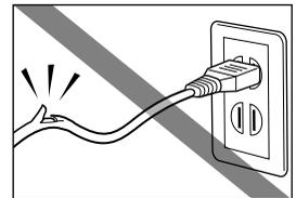
Never plug the printer into a power socket that is shared with other equipment (extension lead, double adapter, etc.).
