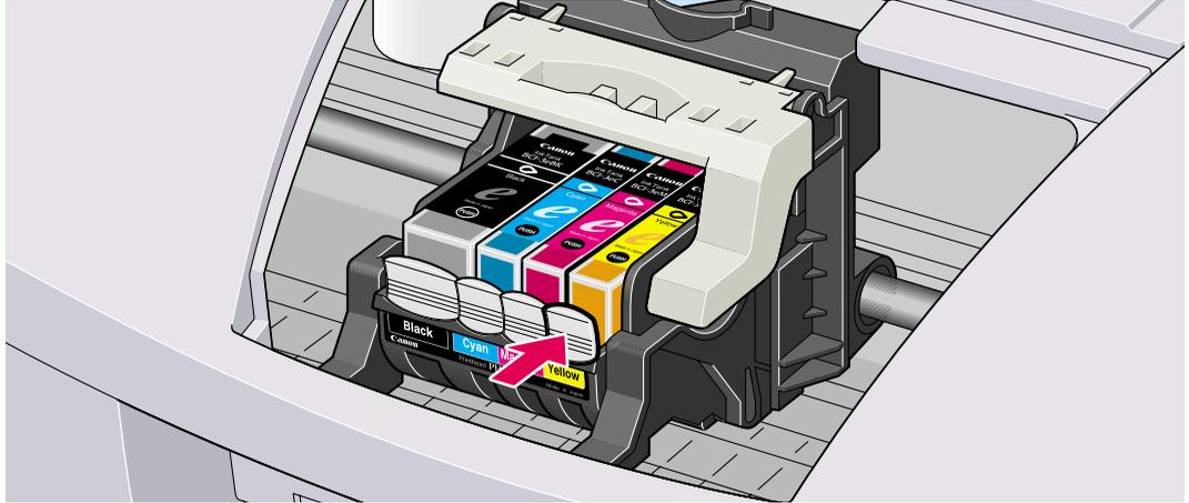
Do not touch the lock lever; remove only the ink tank.
