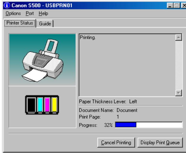
**Note** ➤ To open the BJ Status Monitor when the printer is not printing, click the [Maintenance] tab in the Printer Properties dialog box and click the [Start Status Monitor] button.
