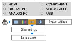
You can reset the lamp counter that indicates the timing to replace the projector when you replace it.
