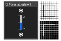
Press the pointer buttons to adjust the focus.
