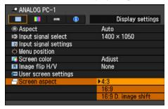
4:3 Select this when you use a screen with aspect ratio of 4:3. You can adjust the keystone distortion with D.SHIFT/KEYSTONE button. 16:9 Select this when you use a screen with aspect ratio of 16:9. You can adjust the keystone distortion with D.SHIFT/KEYSTONE button. 16:9 Select this when you use a screen D. image with aspect ratio of 16:9. You can move the screen upward or shift downward with D.SHIFT/KEYSTONE button.
