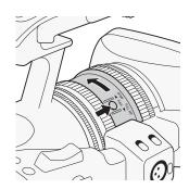
2 Press the PUSH button (unlock focus mode ring button) on the focus mode ring and turn the ring toward AF/MF.
