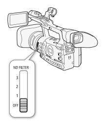
Using the ND filters allows you keep the aperture within an appropriate range when recording in bright surroundings\*.
